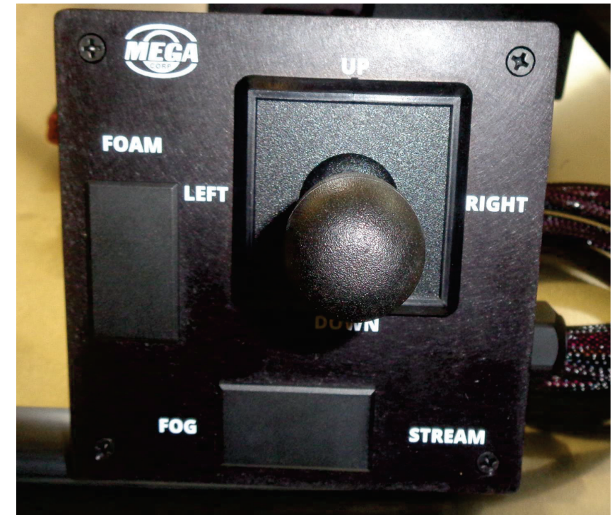
JOYSTICK SHOWN WITHOUT FOAM AGENT AND ADJUSTABLE NOZZLE OPTIONS
